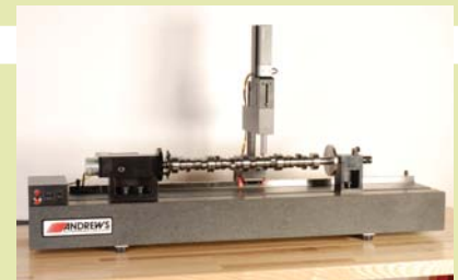
This Andrews Products auto camshaft measurement instrument uses three HEIDENHAIN encoders and a computer interface
