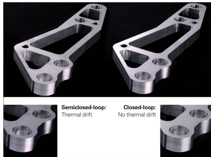
Figure 6 – Coupling lever, processed twice from one blank form
