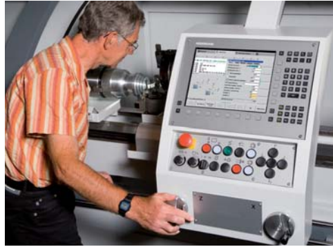
With the MANUALplus 620 both cycle and CNC lathes can effectively be handled
