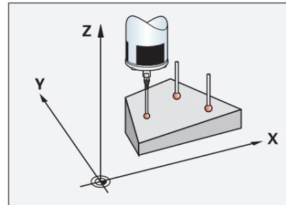
Measuring the angle of a plane
