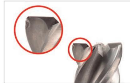
Machining without OCM: Tool after two parts
