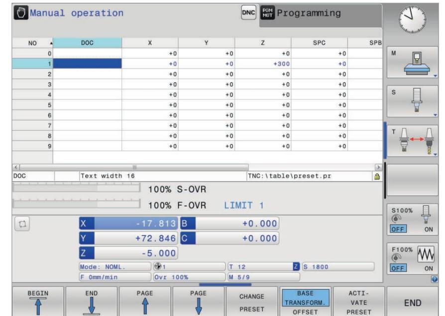
The requirements gap between machining centers and typical tool and moldmaking machines is becoming ever narrower. Of course, the TNC 320 is also very capable of controlling automated manufacturing processes. It features the necessary functionality to manage and measure tools, as well as to inspect the machining process. It helps you reduce non-machining time, increase productivity, and improve production quality.
