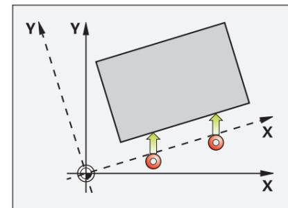
Workpiece misalignment compensated for by rotating the coordinate system or turning the table
